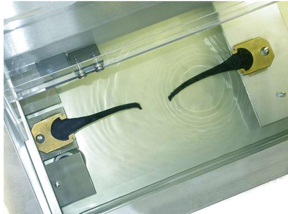
6.2 If the bituminous material comes in contact with the surface of the water or the bottom of the bath, the test shall not be considered normal. Adjust the specific gravity of the bath by using a specific gravity additive as described in Section 4.8 so that the test specimen neither comes to the surface of the water, nor touches the bottom of the bath at any time during the test.
