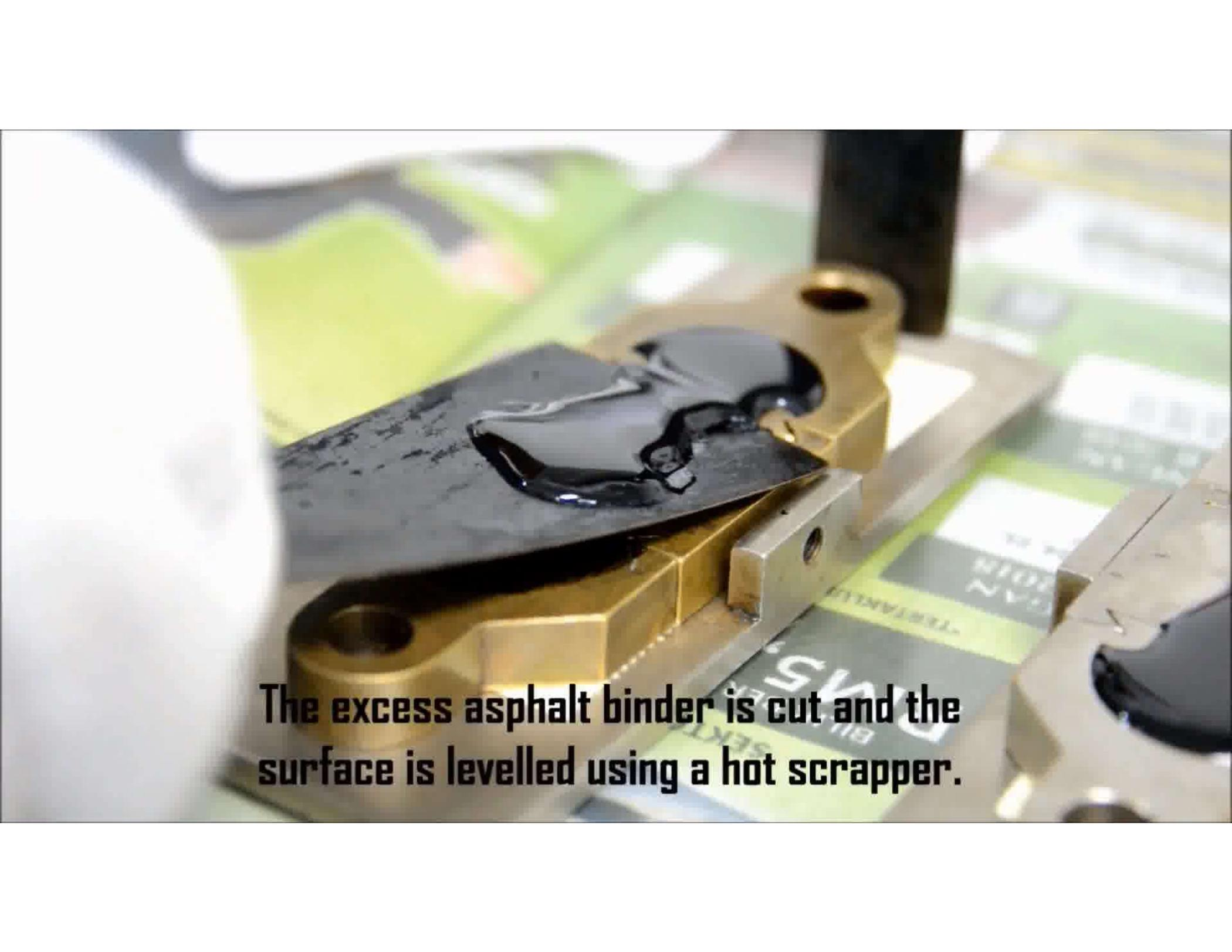
**The excess asphalt binder is cut and the surface is levelled using a hot scrapper.**
