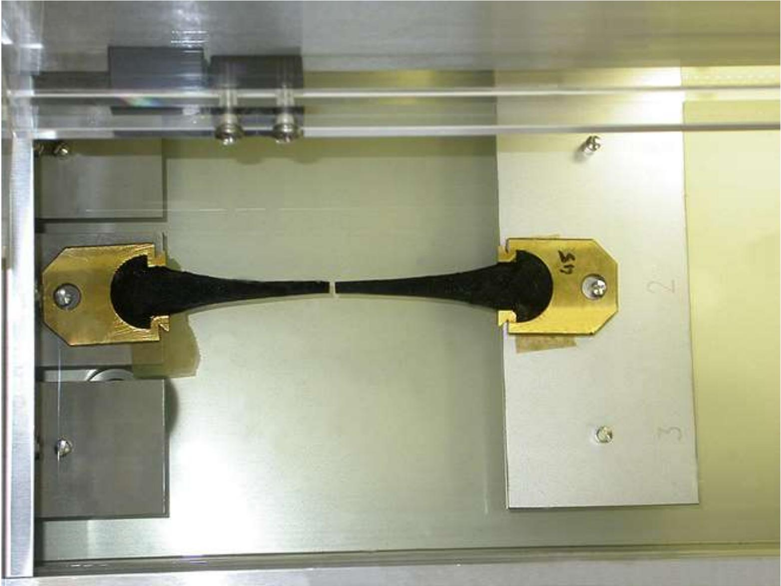
4.2 *Water Bath for Conditioning Specimens*—A water bath capable of maintaining the specified test temperature, varying not more than  $0.5^{\circ}\text{C}$  ( $0.9^{\circ}\text{F}$ ) from this temperature. The specimen shall be immersed and supported such that it is surrounded by water.
