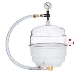
3.2.2 residual pressure, as employed by this test method —the pressure in a vacuum vessel when vacuum is applied.
