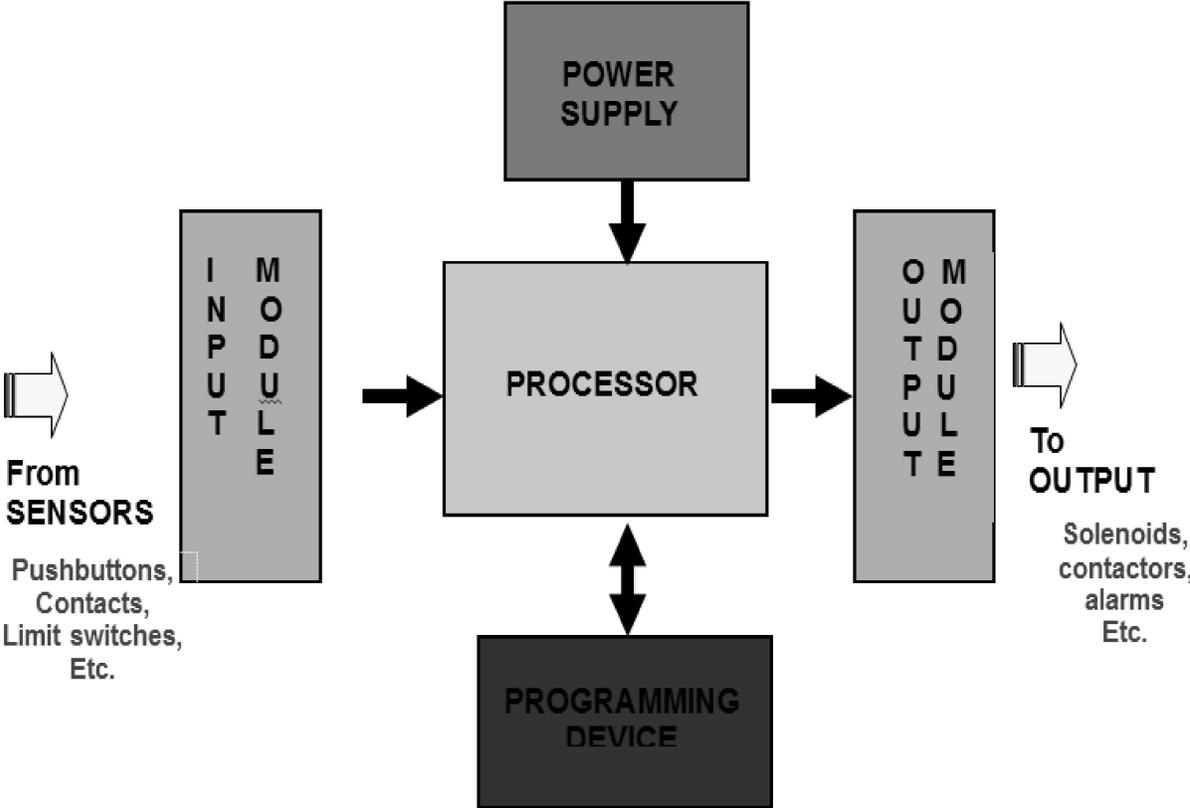
Figure 1: PLC architecture
