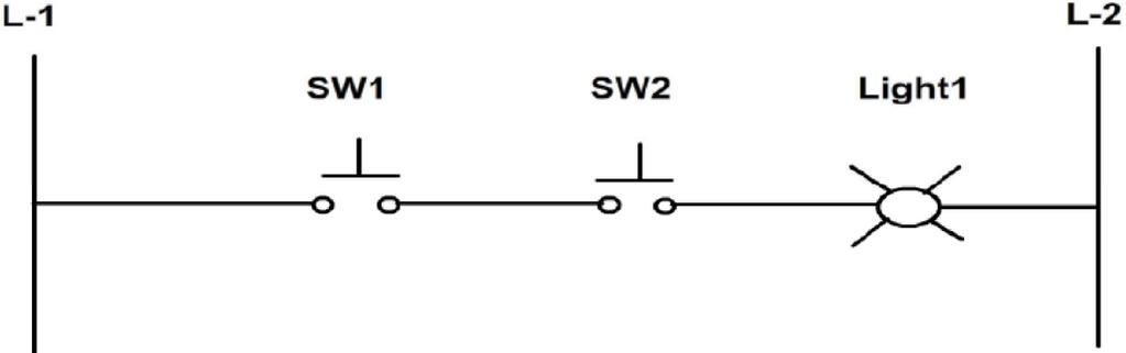
Figure 4: AND-logic function
