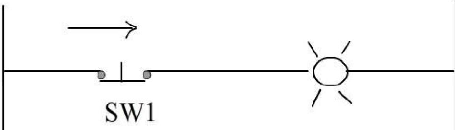
Figure 3: Hardwire switch-lamp circuit
