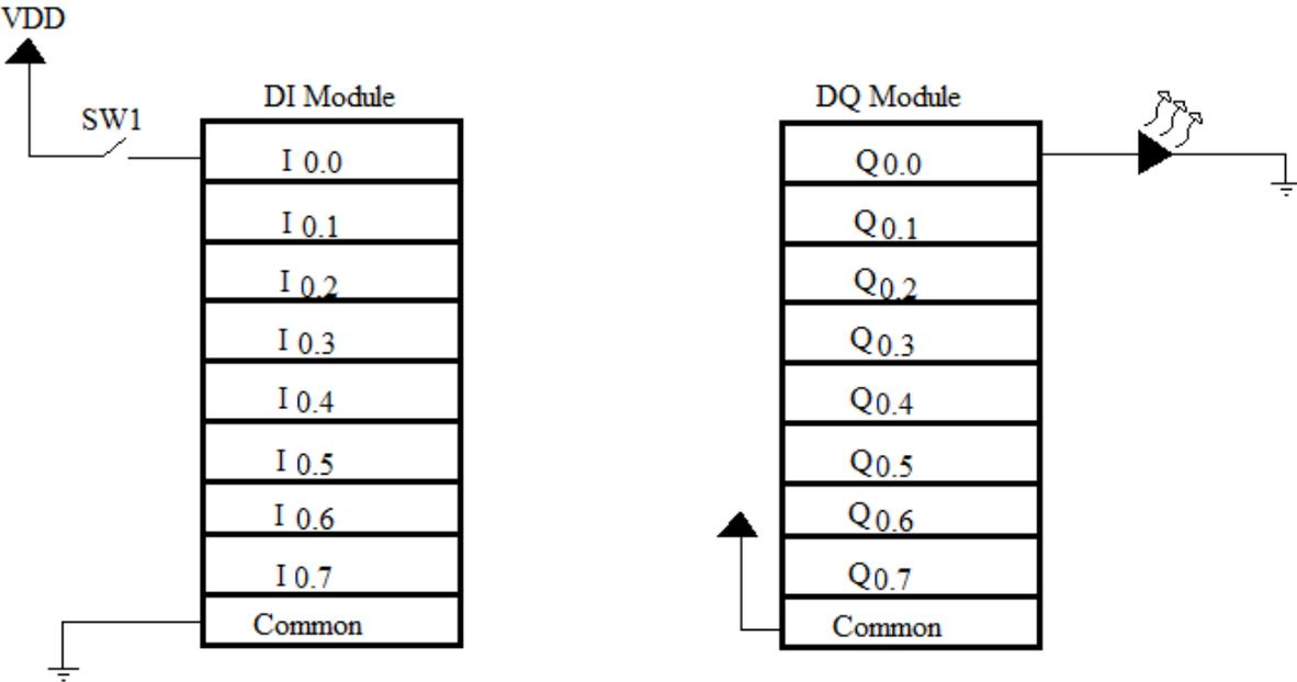
Figure 2: Simple Connection using Siemens S7-400 PLC
