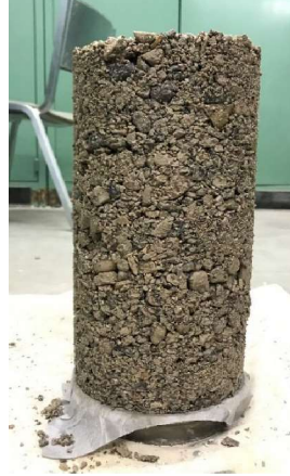
(c) unmolded specimen after compaction
