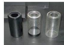
Figure : RTFO Samples (left - after aging in the RTFO, center - before aging in the RTFO, right - empty sample jar)
