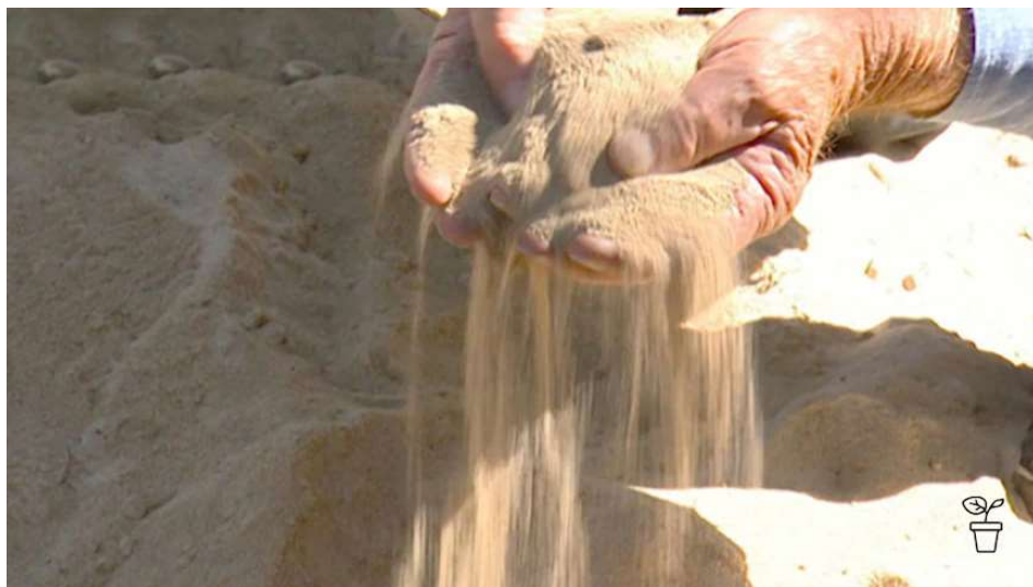
Sand - 2.00-mm (No. 10) to 0.425-mm (No. 40) Sieve
