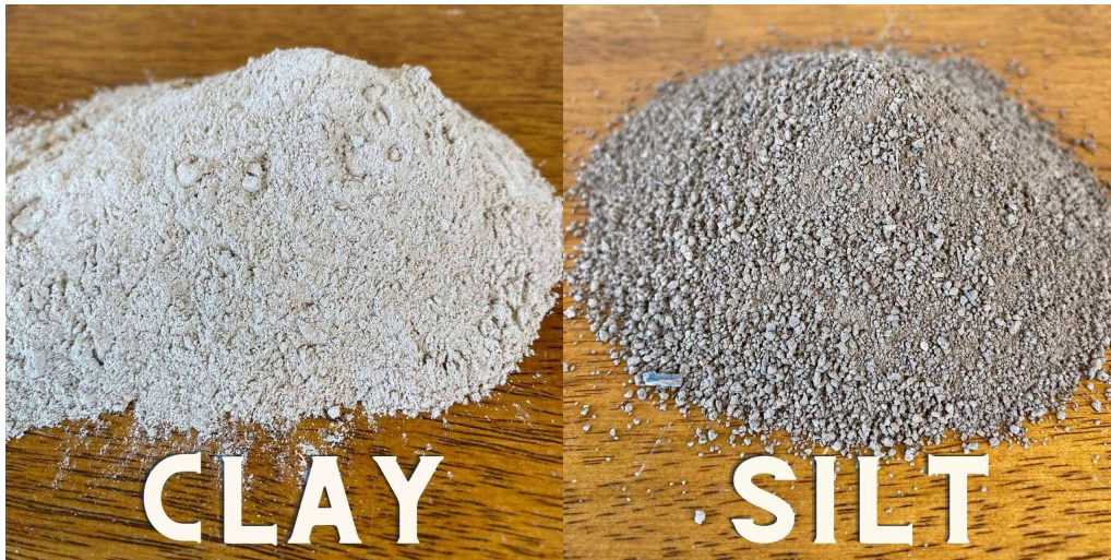
Silt-Clay - Passing 75- \mu\text{m} (No. 200) Sieve
