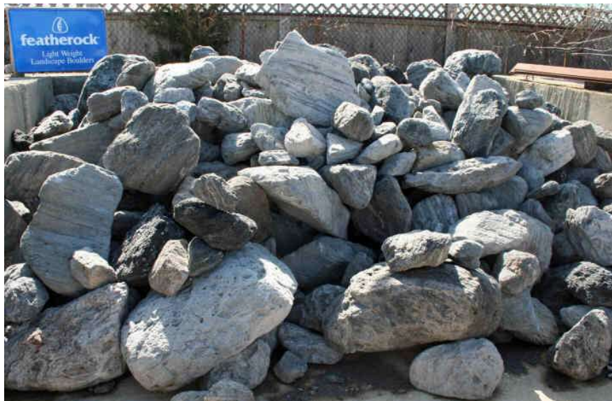
Boulders and Cobbles - Retained on 75-mm (3-in.) Sieve
