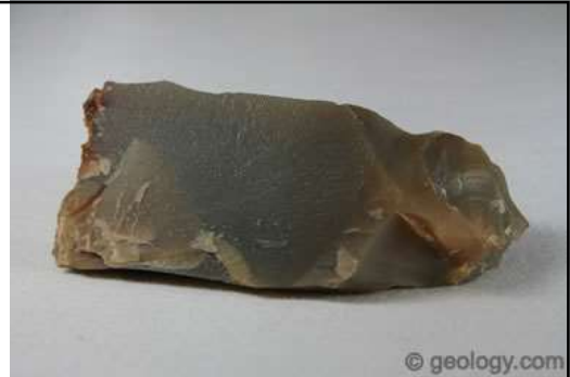
Flint: A specimen of brown, translucent flint from Minas Gerais, Brazil. This specimen has a fine-grained, uniform texture that should perform well in manufacturing tools. Specimen is approximately four inches across.
