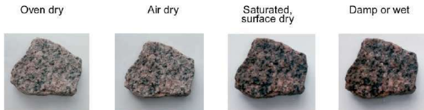
Granite aggregate at various moisture conditions
